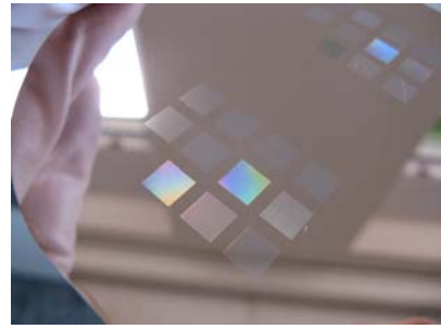
Shim mold inserts in nickel with optical nanostructures
